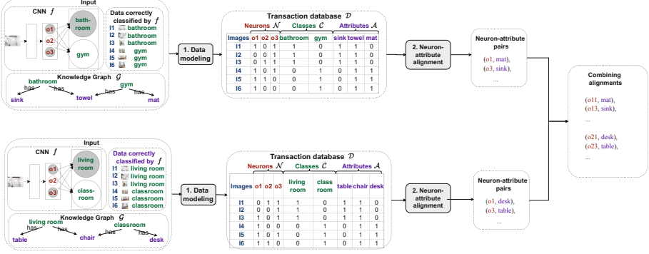
Fig. 4. The figure illustrates how to combine knowledge acquired by two networks. The aggregate alignments are later employed to reason about images from unseen classes.
